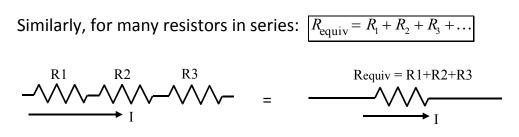
*Important:* the current I is the SAME through each of these series resistors. (What goes in must come out: conservation of charge! This is not an approximation of any kind, it's exactly true)
