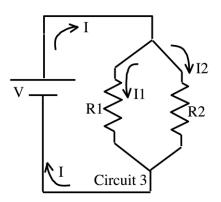
This time, the current I is NOT necessarily the same through R1 and R2.
