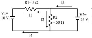
The first step is to draw arrows for currents, and label them. The direction you initially pick for the arrow is arbitrary! It doesn't matter. If you solve for, say, I1 in the picture above, and if it happens to come out negative, that just means the real current is heading the OPPOSITE way from the arrow you drew. (So, it'd be left, in the picture above.)
